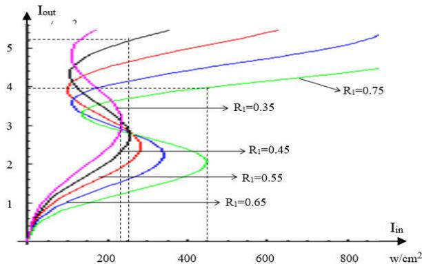
**Figure 2.** Out-input characteristics of SNMI with  $\delta_0 = -0.1\pi$ ;  $L = 1\text{mm}$ ;  $\lambda = 0.85\mu\text{m}$ ,  $R_2 = 0.5$ ;  $n_2 = 10^{-4} \text{ cm}^2/\text{w}$   $L_1 = L/3$ ;  $\alpha = 10^3$  and  $R_1$  change with the values of  $R_1 = 0.35, 0.45, 0.55, 0.65, 0.75$
