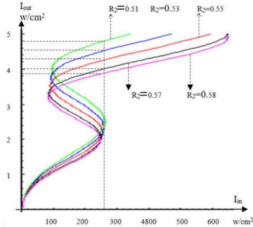
**Figure 4.** Out-input characteristics of SNMI with  $\delta_0 = -0.1\pi$ ;  $L = 1\text{mm}$ ;  $\lambda = 0.85\mu\text{m}$ ,  $R_1 = 0.5$ ;  $n_2 = 10^{-4}\text{cm}^2/\text{w}$ ;  $L_1 = L/3$ ;  $\alpha = 10^3$  and  $R_2$  change with the values of  $R_2 = 0.55, 0.53, 0.51, 0.57, 0.58$
