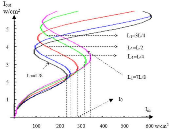
Figure 6. Out-input characteristics of SNMI with  $\delta_0 = -0.1\pi$ ;  $L = 1\text{mm}$ ;  $\lambda = 0.85\mu\text{m}$ ,  $R_1 = R_2 = 0.5$ ;  $n_2 = 10^{-4}\text{cm}^2/\text{w}$ ;  $\alpha = 10^3$  and  $L_1$  change with the values of  $L_1 = L/8$ ;  $L/4$ ;  $L/2$ ;  $3L/4$ ;  $7L/8$
