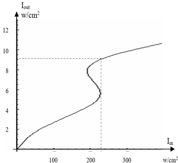
**Figure 3.** Out-input characteristics of SNMI with  $\delta_0 = -0.1\pi$ ;  $L=1\text{mm}$ ;  $\lambda = 0.85\mu\text{m}$ ,  $R_2 = 0.5$ ;  $n_2 = 10^{-4} \text{ cm}^2/\text{w}$   $L_1=L/3$ ;  $\alpha=10^3$  and  $R_1 = 0$
