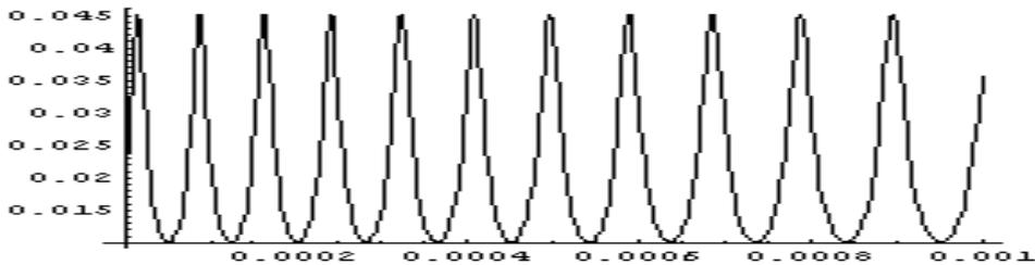
Figure 7. The dependence of the "Transfer Function" ( $F = I_{out} / I_{in}$ ) on the position of the input light ( $L_1$ ). With  $\delta_0 = -0.1\pi$ ;  $L = 1\text{mm}$ ;  $\lambda = 0.85\mu\text{m}$ ,  $R_1 = 0.45$ ;  $R_2 = 0.5$ ;  $n_2 = 10^{-4}\text{cm}^2/\text{w}$ ;  $\alpha = 10^3$  and  $I_{out} = 100\text{w/cm}^2$
