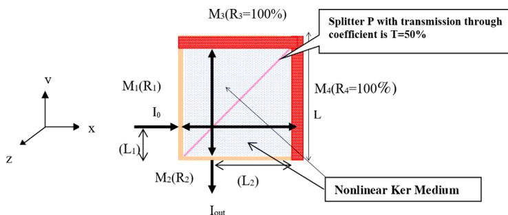
**Figure 1.** *Symmetric Nonlinear Michelson Interferometer*
