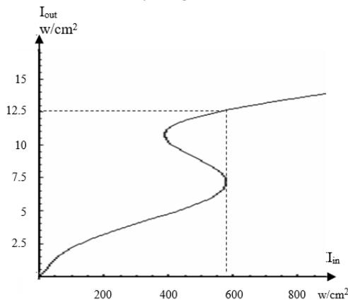
**Figure 5.** Out-input characteristics of SNMI with  $\delta_0 = -0.1\pi$ ;  $L = 1\text{mm}$ ;  $\lambda = 0.85\mu\text{m}$ ;  $R_1 = 0.75$ ;  $n_2 = 10^{-4}\text{cm}^2/\text{w}$ ;  $L_1 = L/3$ ;  $\alpha = 10^3$  and  $R_2 = 0$
