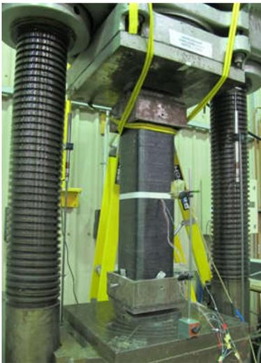
**Figure 10.** Strengthening rectangular columns with hoop FRP sheets
