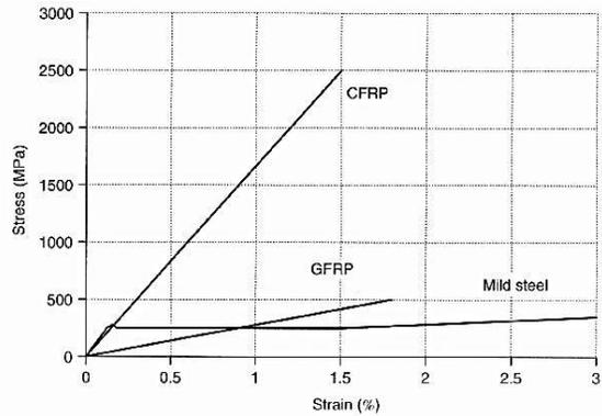
Figure 2. Typical FRP and mild steel stress-strain curves
