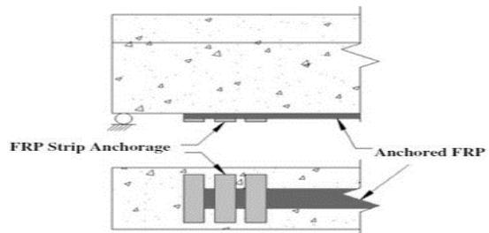
**Figure 6.** FRP strip anchorage
