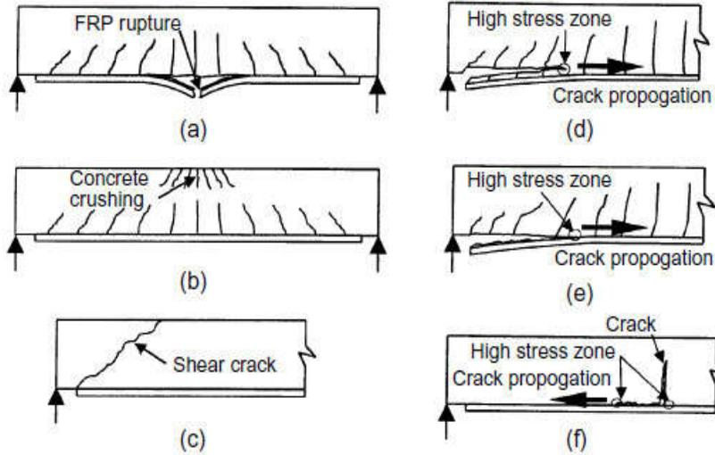
**Figure 4.** Failure modes of strengthened beams
